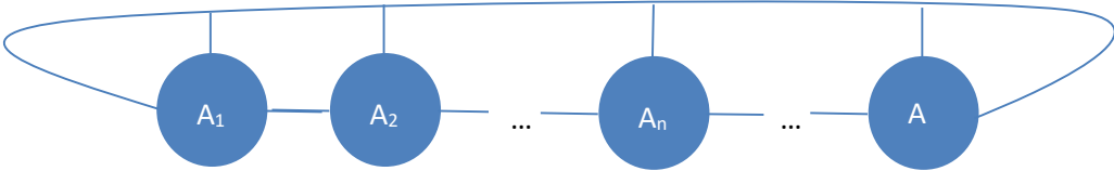
Figure 11: Tensor Ring Illustration showing that only order-3 core tensors are used and connected circularly.
